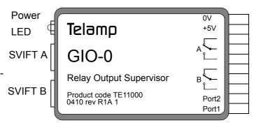
GIO0 is a very simple supervisor for SVIFT equipment, indicating alarm status in any of the connected units by activating its relays. Up to 8 units can be supervised, connected to both or one of its SVIFT interface jacks, as separate chains or in a loop configuration. It scans all connected units for ROFLB objects and handles its output relays according to the A- or B-alarm determined by these. It also optionally can handle the LEDs on the connected units to identify which unit causes the alarm.
