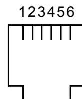
All cables are 2\*2 twisted pairs shielded 0.14 - 0.23 mm<sup>2</sup>, using 1-2 as one pair and 3-4 as the other. All cables have pins 2 and 4 “crossed”, i.e. has pin 2 at one end connected to pin at the other 4 and vice versa. Pins 1 and 3 are always “straight” connected, i.e. matching pin numbers connected.
